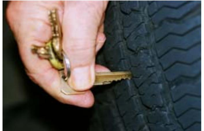
**Photo 6 – Tire Tread Depth:** Measure. 11/32 inch is new condition on most tires. 2/32 inch is worn out (wear indicator depth).
