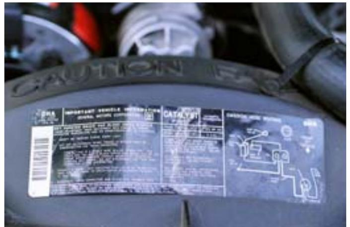
**Photo 4 – Read the Label:** Follow correct procedures and adjust to specified base timing.
