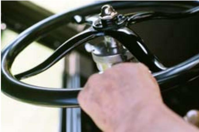
**Photo 5 – Steering Freeplay:** Wiggle steering wheel to test “freeplay.” One inch is normal. Inspect for excess clearance in steering mechanisms. **See Text.**
