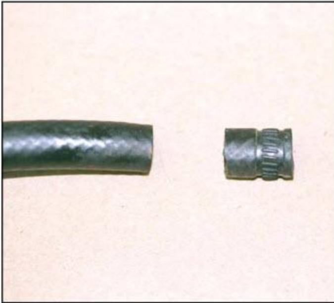
PHOTO 1 - Fuel Line Service: If the old fuel line is cracked on the outside or mushy on the inside, replace the fuel line with the correct size SAE rubber tubing [no 5/16 on a 1/4 inch line]. Install clamp. Do not cut surface.
