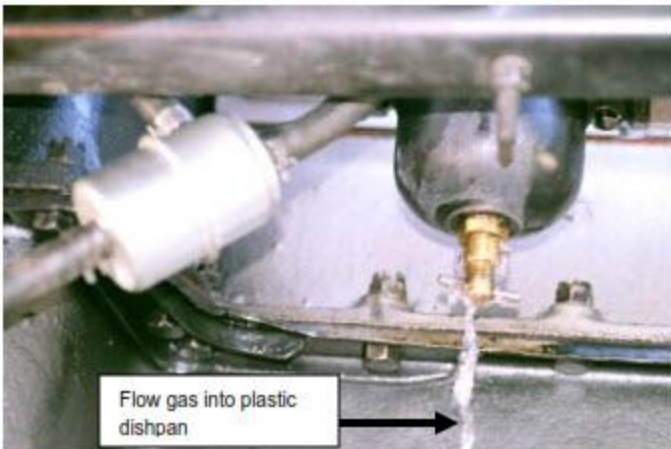
PHOTO 3 – Fuel Flow Check, Needle Valve: Check fuel flow by opening the carburetor drain. This will flush needle and seat. Drain into plastic dishpan.
