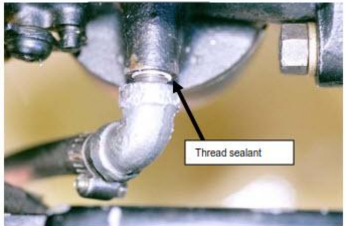
PHOTO 4 – Fuel Line Sealant: Use Permatex sealant on pipe threads. Apply sparingly. Never, never use Teflon Tape.
